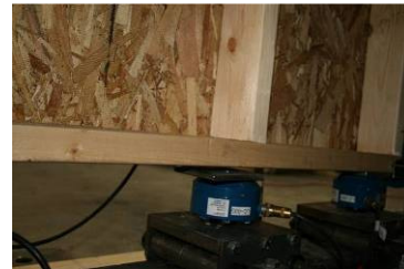
Photo 32: Base Bearing Plate
