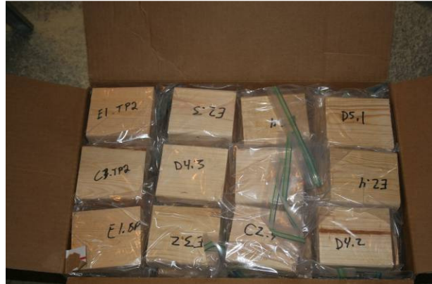
Photo 44: Specific Gravity Samples from Wall Specimens
