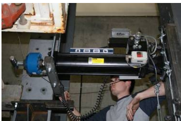
Photo 35: Alignment of Horizontal Actuator
