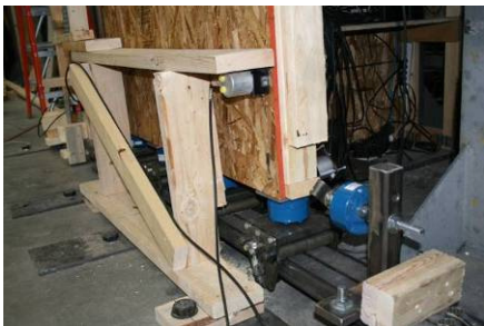
Photo 43: String Potentiometer Connection
