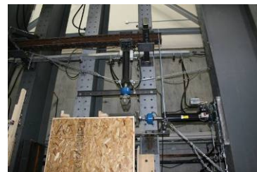
Photo 36: Restraint of Actuators
