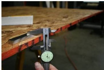
Photo 8: Thickness of OSB
