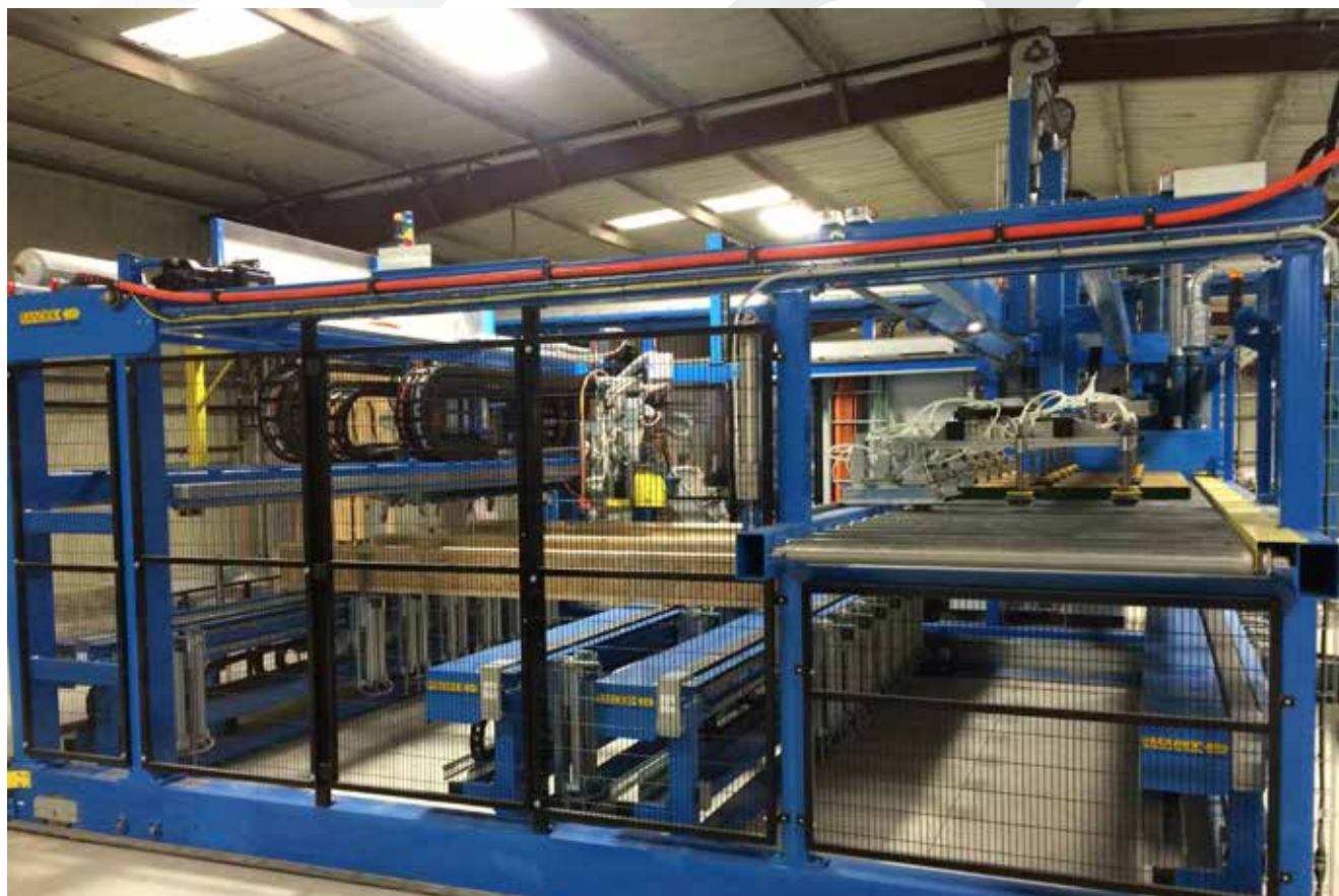
AutoFloor bridge working over jig system: gluing, adding sheets, handling tongue and groove connection, stapling/nailing, sawing, milling and marking using inkjet
