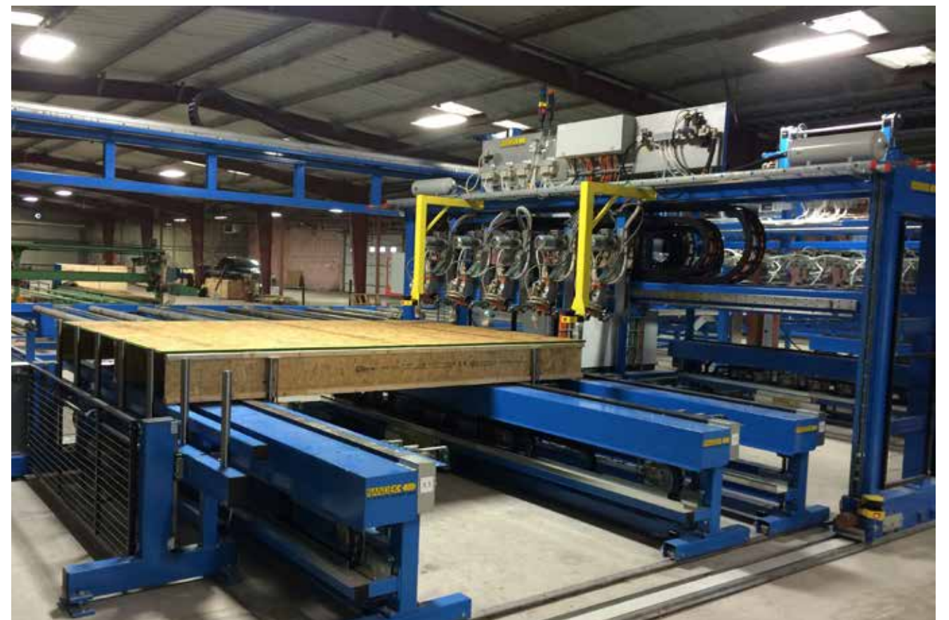
AutoFloor bridge positioned next to AutoFloor jig system
