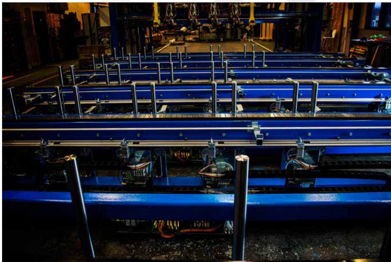
Empty AutoFloor jig with pins activated/upraised
