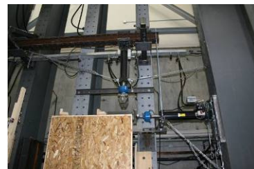
Photo 36: Restraint of Actuators
