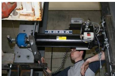
Photo 35: Alignment of Horizontal Actuator
