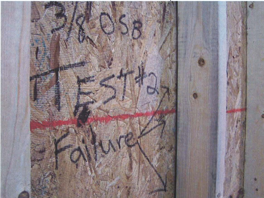
Test #2 3/8" OSB - Failure
