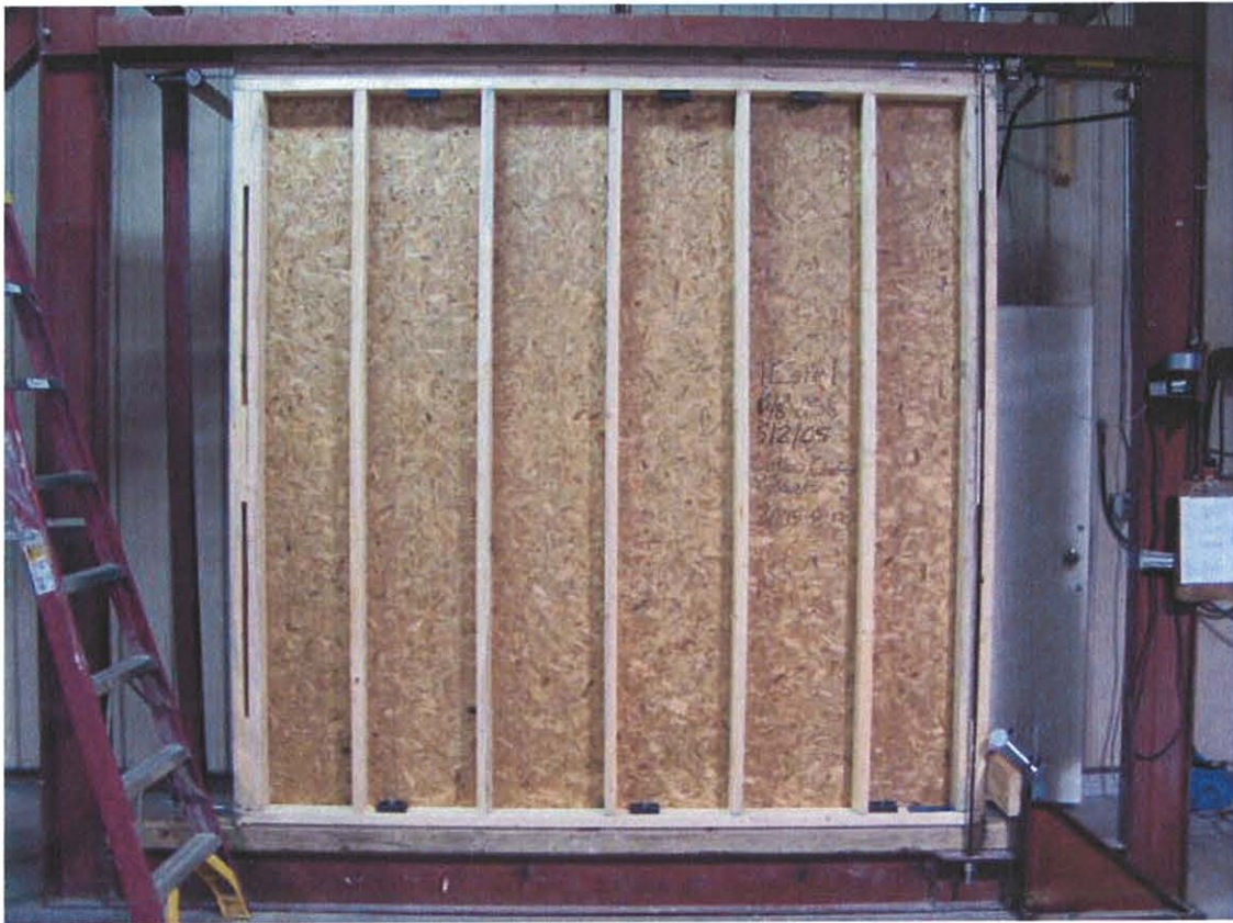
Test #1 3/8" OSB - Set-up
