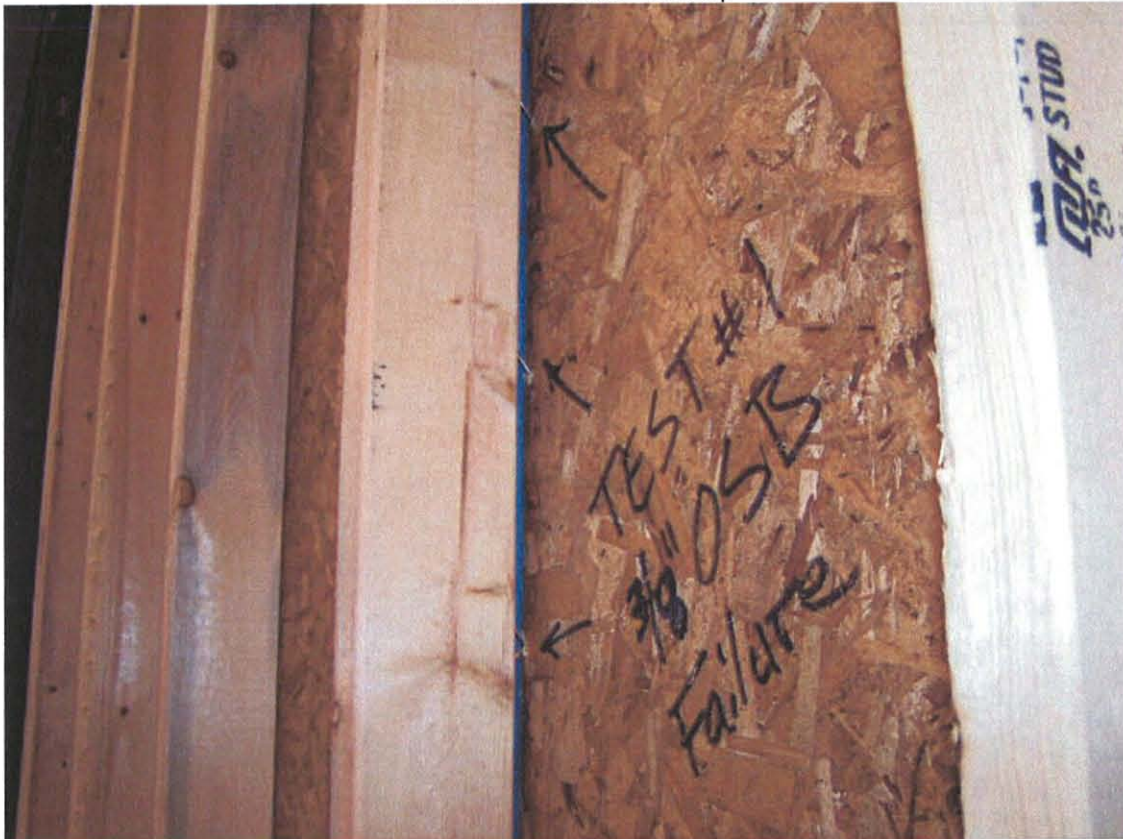
Test #1 3/8" OSB - Failure
