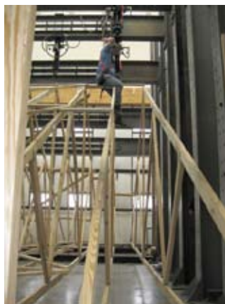
SBCRI lab staff members were used to simulate loads on A2.
