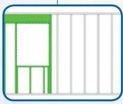
Create portal frames quickly fo APA braced wall (shear panel) requirements
