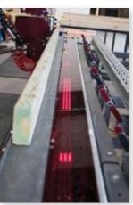
The MiTek 16' long Light Bar is the latest edition to our wall panel equipment package. It indicates the starting point for the wall, and the location of subcomponents, corners and specials, eliminating marking errors and decreasing layout time in your wall panel plant. This labor-saving tool is driven by our ShopNet™
