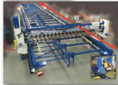
• Custom built 95 feet of expanded wall panel capability with Dual Tool Beam and Dual Top & Bottom Nailers (builds up to 76' wall)
