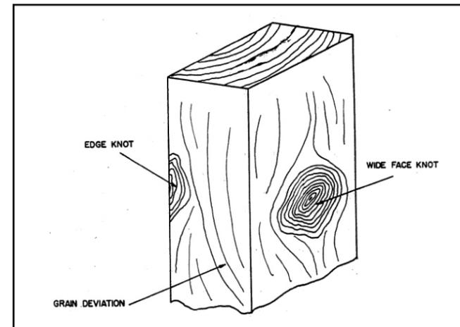
Figure 1. Sketch depicting knots and grain deviation in lumber.
