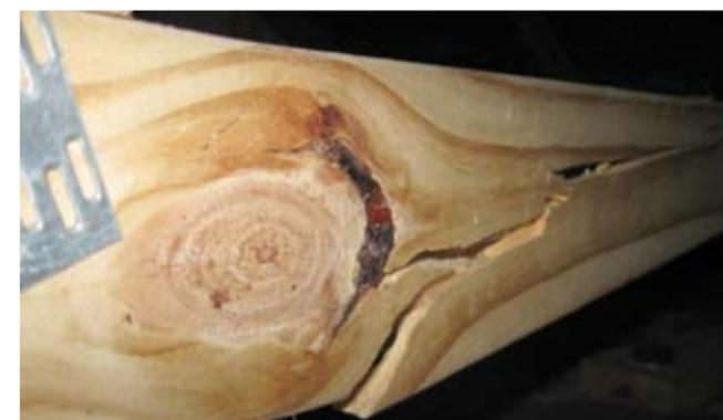
Figure 2. Failure in bottom chord of truss initiating in grain deviation around large wide face knot.
