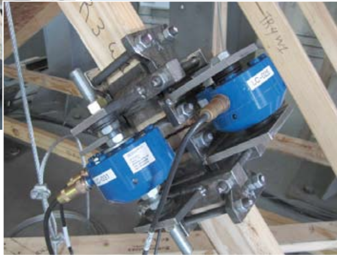
Figures 11 & 12. WB3 is used to test the forces through a web in a full-scale assembly.
