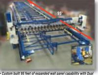
Custom built 95 feet of expanded wall panel capability with Dua Tool Beam and Dual Top & Bottom Nailers (builds up to 76' wall)
