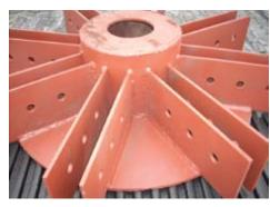
Additionally, Kennedy came up with the concept to use steel compression and tension rings to tie the trusses into, and worked with a local engineer to design them. "There's a ring located at the top and bottom chord connections to handle both gravity and wind loads," he said. A local certified welder custom made the rings. (See photo at left.)
