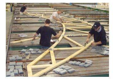
This month's shots come from loyal submitter Chris Lenauer of Pioneer Truss Company. The trusses being built at left are double radius, meaning both the bottom and top chords are curved.
