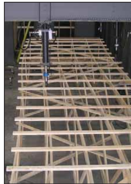
Photos 4 & 5. In order to make this testing possible, once the foundation was set, each truss was manually distorted into an "S" shape to imitate the trusses installed in the building, and then braced to retain that shape.
