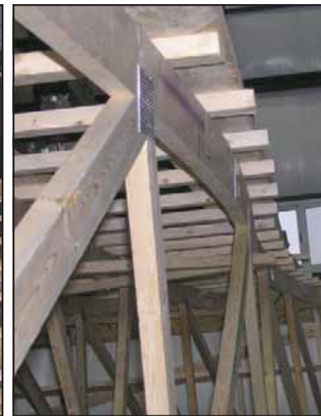
Photos 4 & 5. In order to make this testing possible, once the foundation was set, each truss was manually distorted into an "S" shape to imitate the trusses installed in the building, and then braced to retain that shape.
