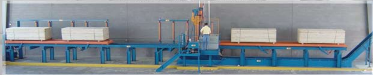
The Verticut P4 System will process three 8 foot bundles of lumber to P.E.T. stud length in less than 13 minutes
