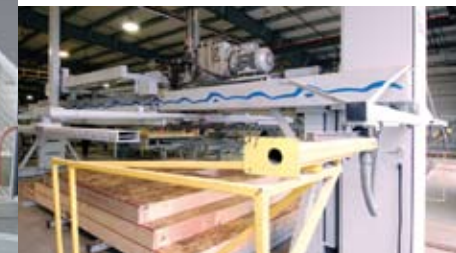
Automated Panel Stacker
