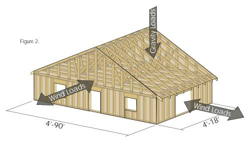
In all the testing combinations we will be able to apply loads simultaneously in vertical (gravity and uplift and cyclical) and horizontal planes (parallel and perpendicular to roof framing and cyclical).
