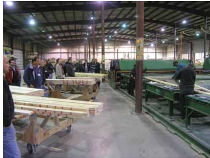
Tour participants watch as John Mulligan talks about assembling trusses on the gantry table at the Saratoga Lumber Traders (SLT) plant in Ballston Spa, NY.
