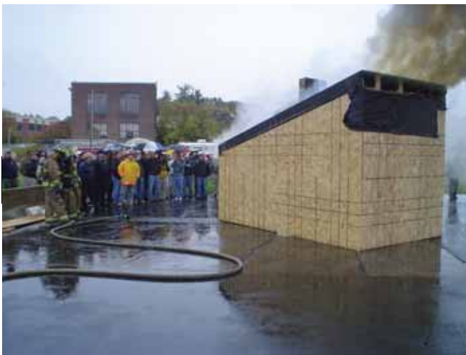
280 firefighters and building officials attended. The observers were asked how long they thought the joists would last in the fire, and how long the trusses would last. Many thought the trusses would fail much sooner.
