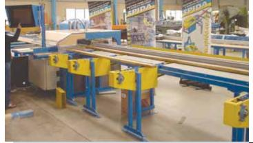
Live deck infeed – operator simply loads the lumber and removes the cut components from the outfeed bench.
