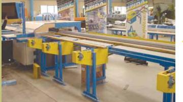
Live deck infeed – operator simply loads the lumber and removes the cut components from the outfeed bench.
