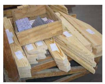
A box on top of cut webs contains the precise number of connector plates for that specific truss.
