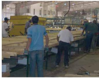
Lumber is placed on a table in preparation for the headers to be nailed.
