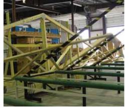
A vertical truss stacker aids in finished product handling on Blenker's new roof truss line.
