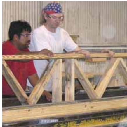
Two first shift production workers from the wood truss shop assemble a floor truss.
