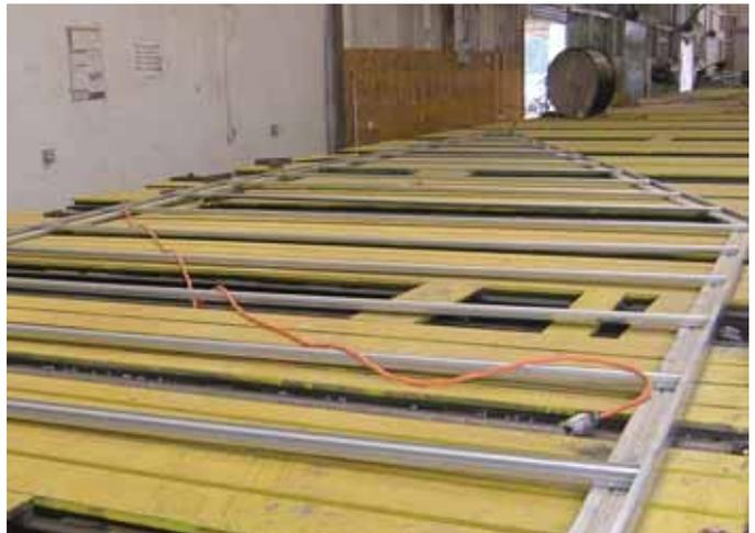
A steel gable end sits on a table in the steel shop. Bama's wood and steel manufacturing operations are housed in separate buildings and there is no cross-over of production staff.
