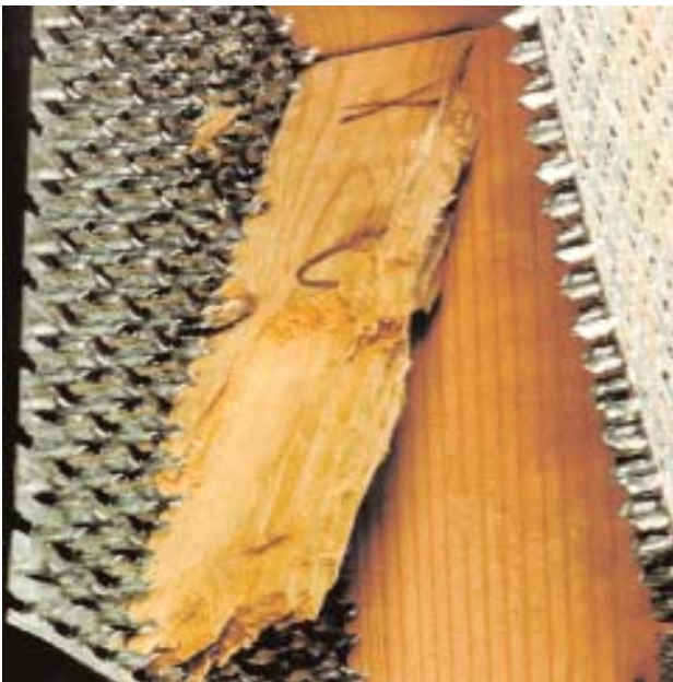
Photo of test joint after chunk-out failure in web.
