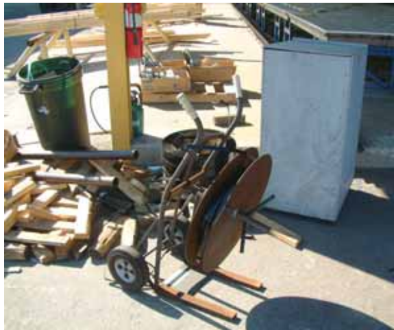
Before: Messy pile of scrap and banding blocks the walkway and creates a potential tripping hazards.
