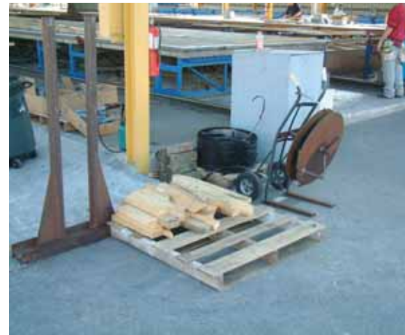
After: Neat stack of scraps with banding put away makes for easy garbage removal and safe vicinity.
