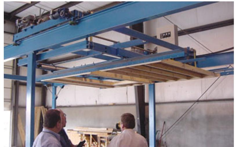
ABC'S NEW CRANE AUTOMATICALLY STACKS EACH PANEL AS IT IS ROLLED OUT OF THE END OF THE ASSEMBLY LINE.
