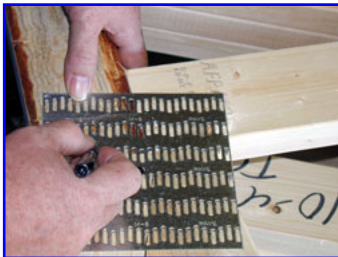
FIGURE 5. EFFECTIVE TOOTH COUNTS NOW CONSIDER BOTH PLATED FACES.
