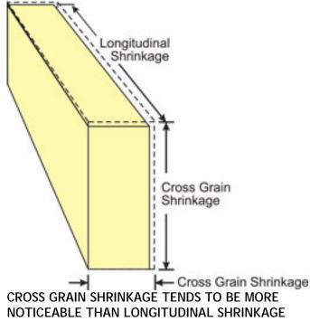
Lumber shrinks as it dries from its fiber saturation point (28 to 30 percent MC) to the moisture level of the surrounding atmospheric conditions (equilibrium moisture content [EMC]). In the Continental U.S., the EMC level is between eight and 12 percent. Therefore, even if kiln-dried lumber is used, there will be some type of lumber shrinkage as the MC drops from about 19 percent to about ten percent.
