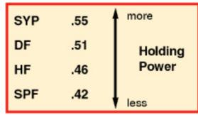
Figure 2. Specific Gravity (G)
