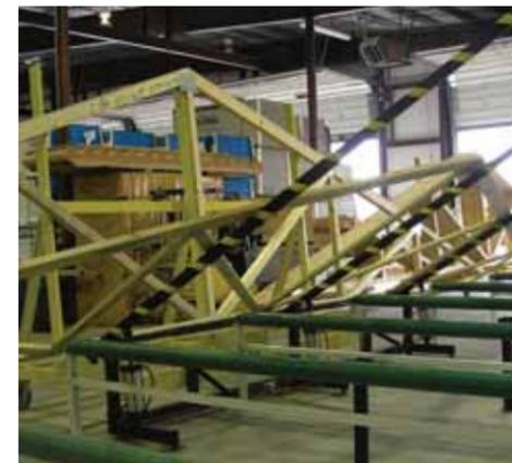
A vertical truss stacker aids in finished product handling on Blenker's new roof truss line.
