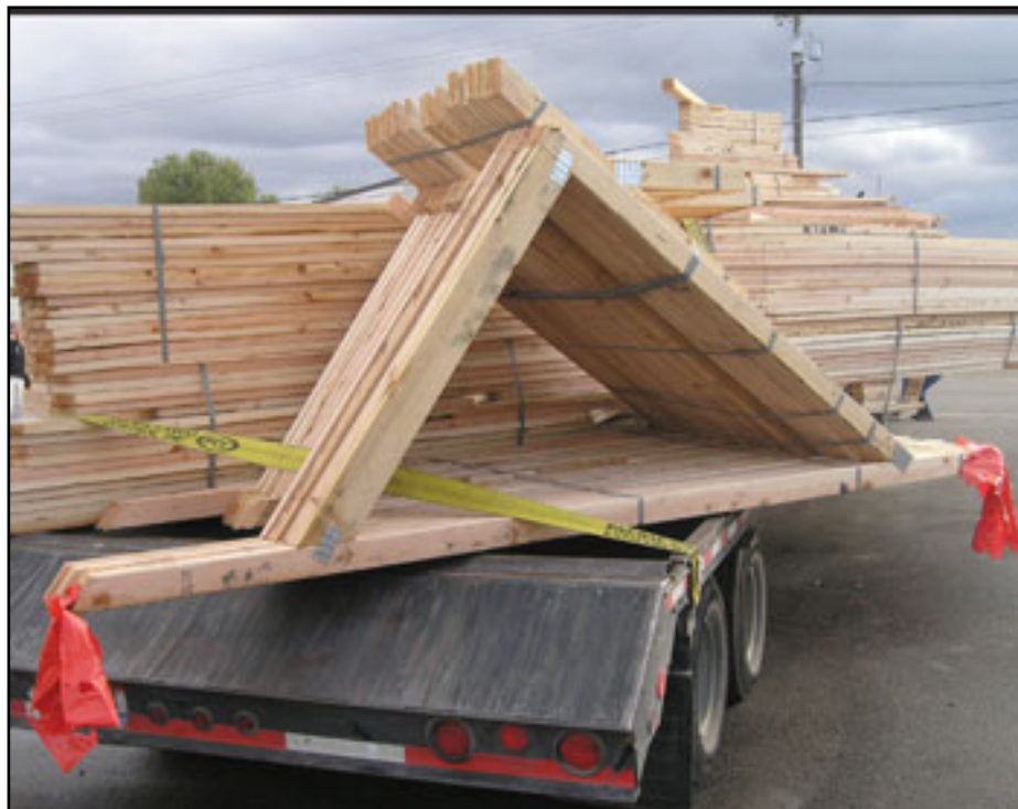
IN THE CASE OF OVERHANGS, EITHER OR THE FRONT, REAR OR SIDE OF THE VEHICLE, MOST STATES REQUIRE PLACEMENT OF FLAGGING AND OTHER CAUTIONARY SIGNAGE ON THE OUTERMOST EDGE OF THE MATERIAL.
