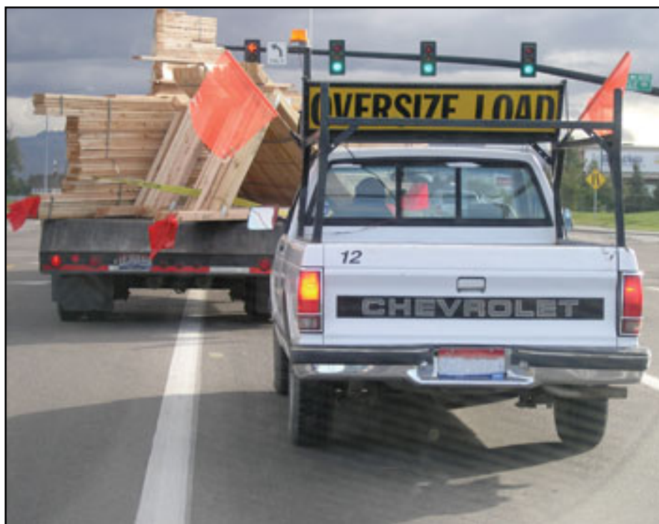
REQUIREMENTS FOR ESCORT VEHICLES VARY BY STATE. IN GENERAL, MOST PERMITS AT THE TIME OF ISSUANCE WILL INDICATE IF, AND HOW MANY, ESCORT VEHICLES ARE REQUIRED FOR THAT PARTICULAR LOAD.
