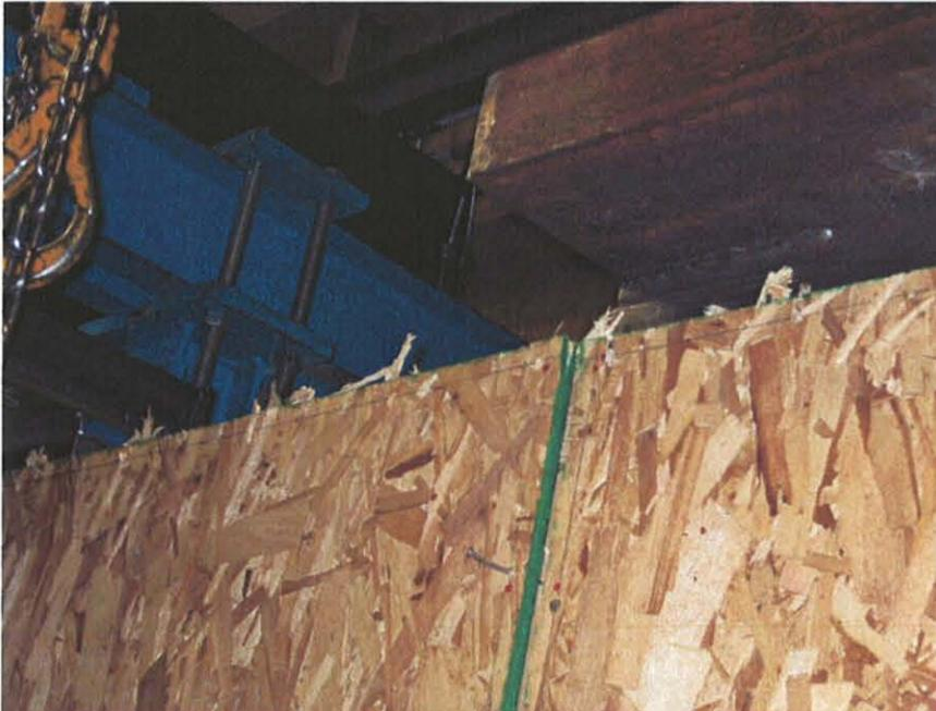
**Figure 8:** Typical OSB sheathing edge tearout
