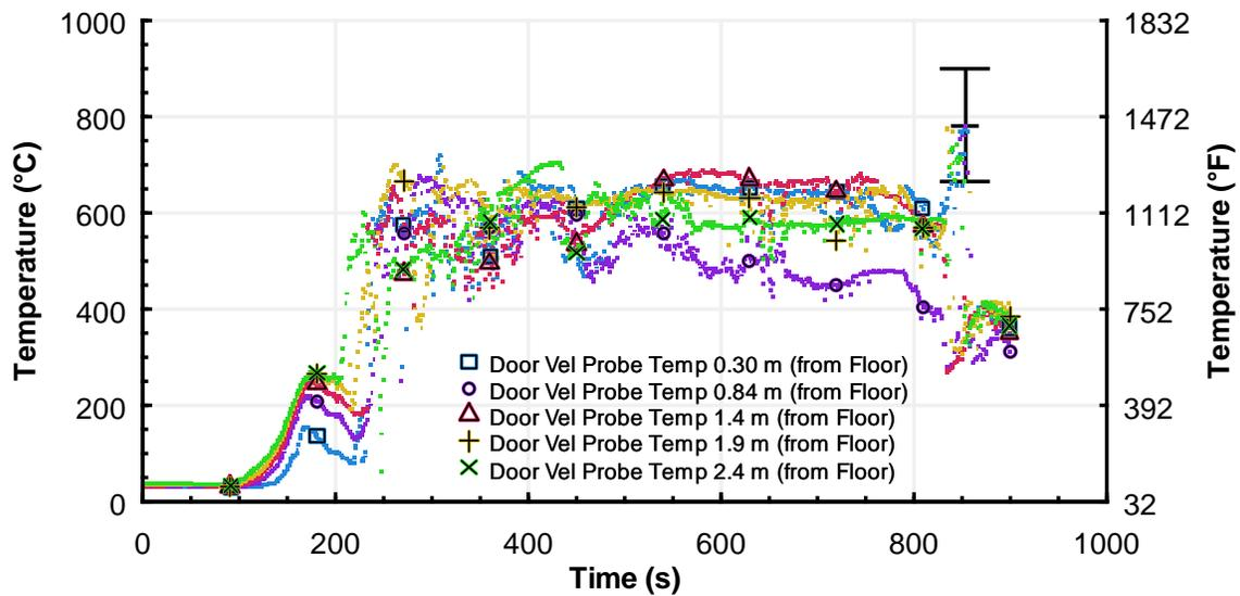
Figure 23. Temperature profile of the thermocouples attached to the bidirectional probes at the top of the basement stairs in the bungalow experiment 4.
