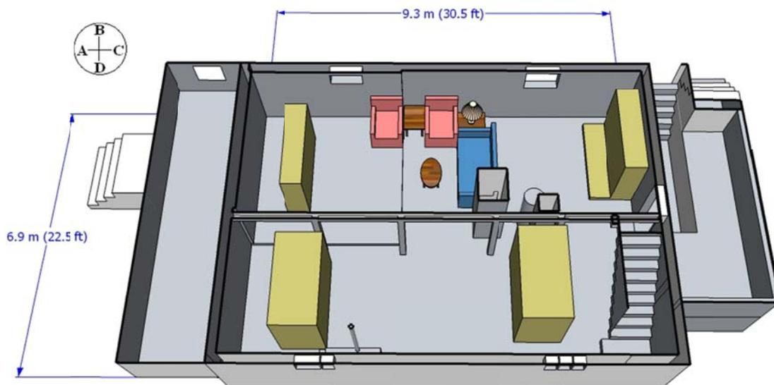
Figure 20. Floor plan of basement with fuel package locations.
