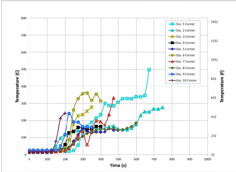
Figure 44. First floor corner temperatures 3 ft. above the floor
