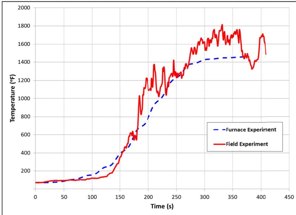
Figure 35. Temperature Comparison for Span Analysis of Engineered I-joist Experiments
