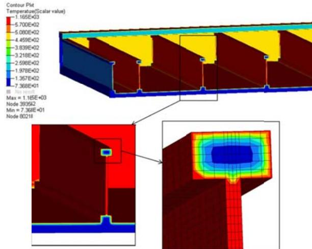
**Figure 24. Temperature contours for engineered wood I-joist supported floor**
