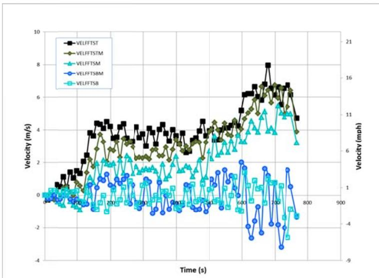
Figure 40. Field Experiment 2 Velocities at the top of the stairs
