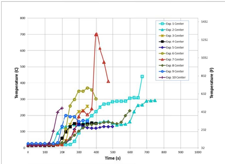
Figure 43. First floor center temperatures 3 ft. above the floor
