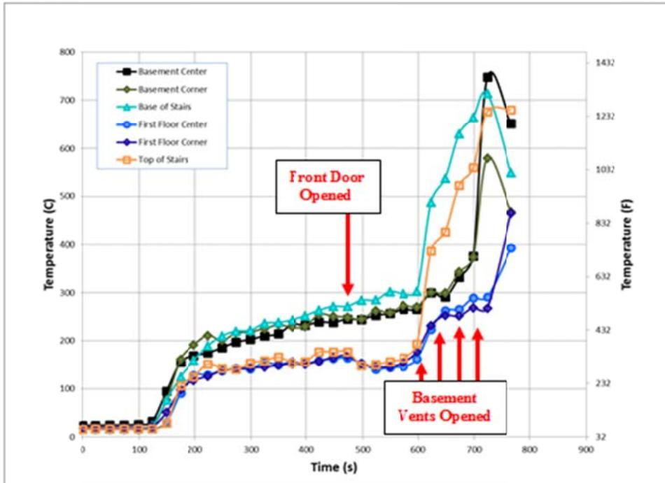
Figure 39. Field Experiment 2 Temperatures at 3 ft. above the floor
