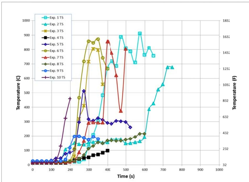
Figure 45. First floor stair temperatures 3 ft. above the floor
