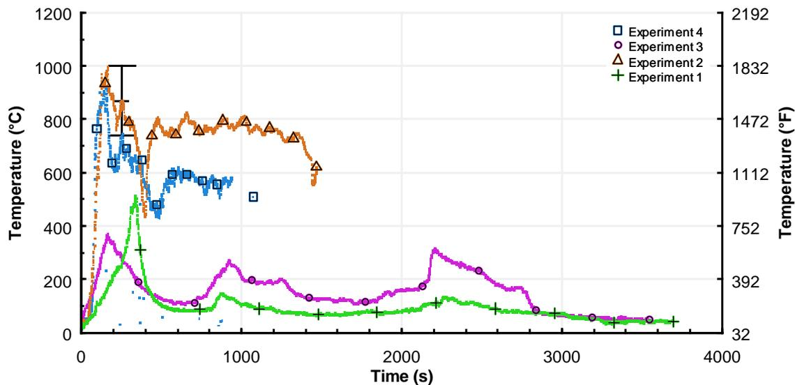
**Figure 21. Temperature at 30 cm from ceiling at the side B location for each experiment.**
