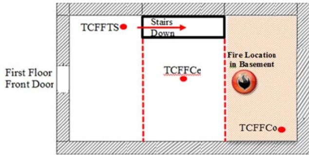
Figure 42. First floor temperature locations and collapse zone
