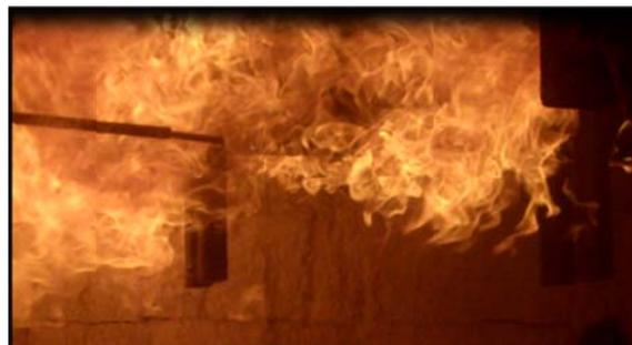
**Figure 10. Image from video of flaming of web for I-joist fire test**
