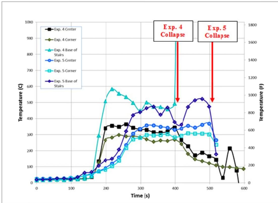
Figure 32. Basement temperatures at 6 ft. above the floor for Experiments 4 and 5
