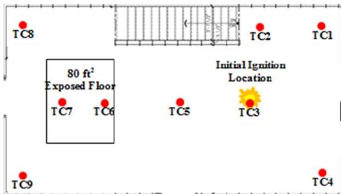
Figure 58. Experiment D Void Thermocouple and Exposed Floor Location
