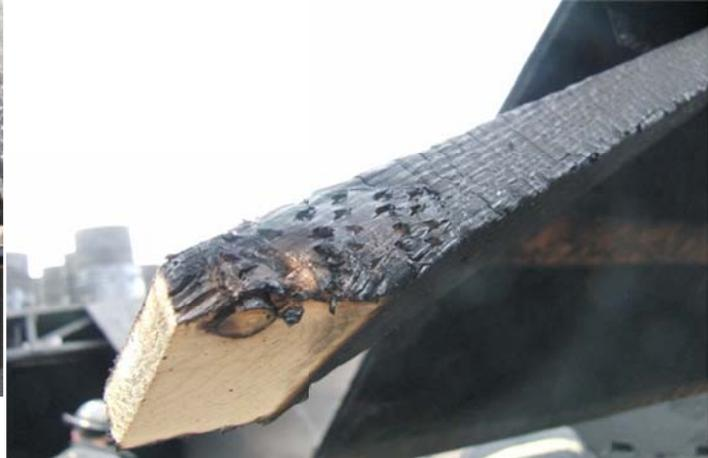
**Figure 51. MPCWT Detail of Connection Failure**
