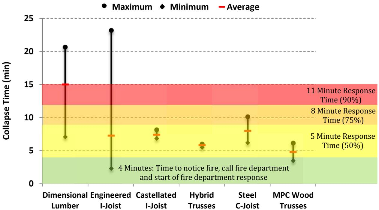
Figure 36. Collapse times versus fire department response times
