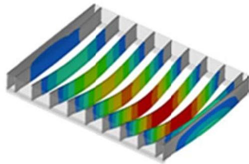
Figure 8. Finite Element Model of an Engineered I-joist Floor System
