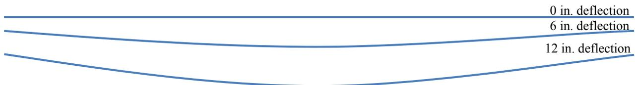
**Figure 41. Relative depiction of 0, 6 and 12 in. deflections on a 20 ft. span**
