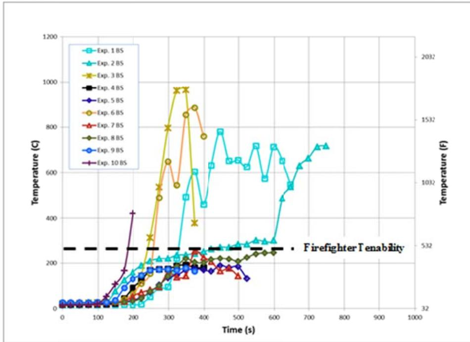
Figure 38. Field Exp. Temperatures 3 ft. above the floor at the bottom of the stairs
