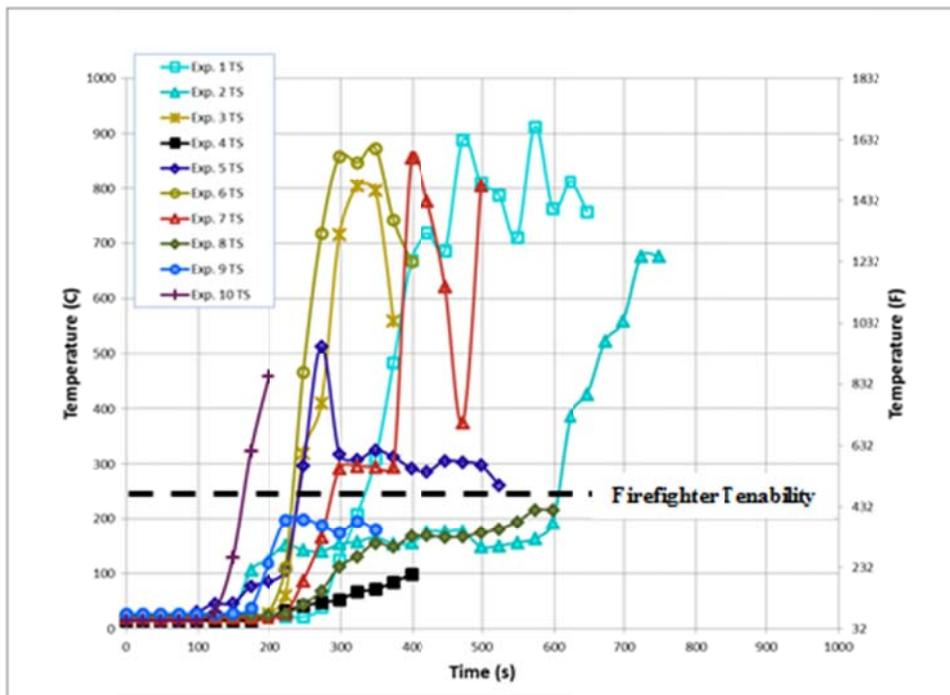
Figure 37. Field Exp. Temperatures 3 ft. above the floor at the top of the stairs
