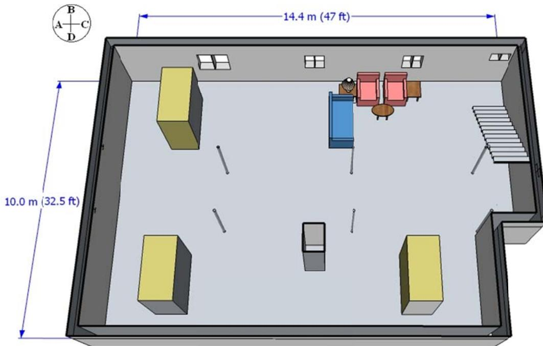
Figure 18. Floor plan of basement with fuel package locations.
