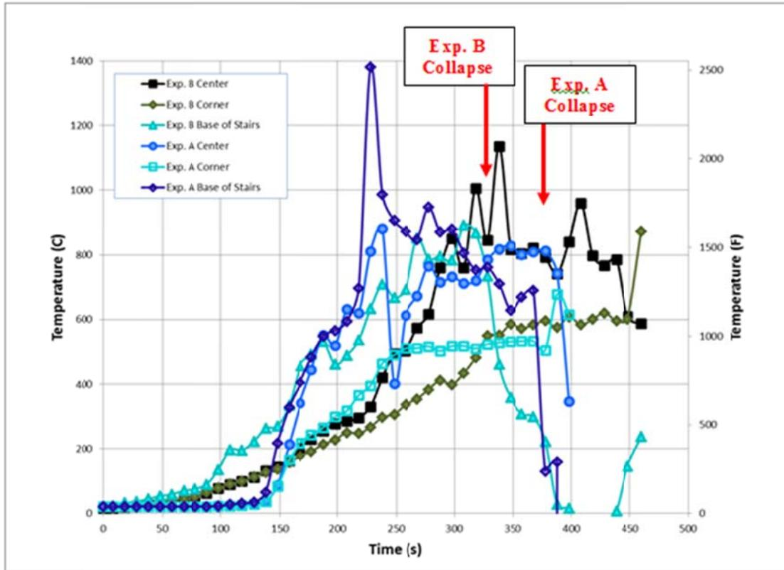
Figure 33. Basement temperatures at 6 ft. above the floor for Experiments A and B
