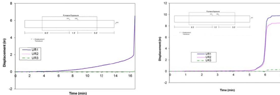
**Figure 9. Deflections for traditional lumber beam (left) and engineered wood I-joist (right)**
