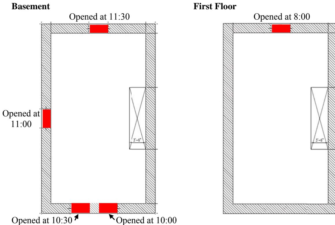
**Figure 31. Sequenced Ventilation Details**
