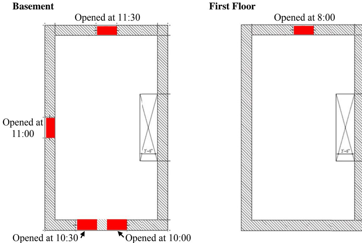
**Figure 31. Sequenced Ventilation Details**
