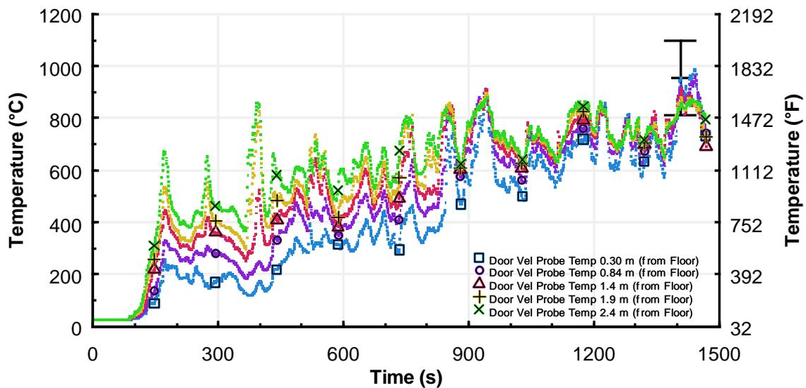
**Figure 22. Temperature profile of the thermocouples attached to the bidirectional probes at the top of the basement stairs in the colonial experiment 2.**
