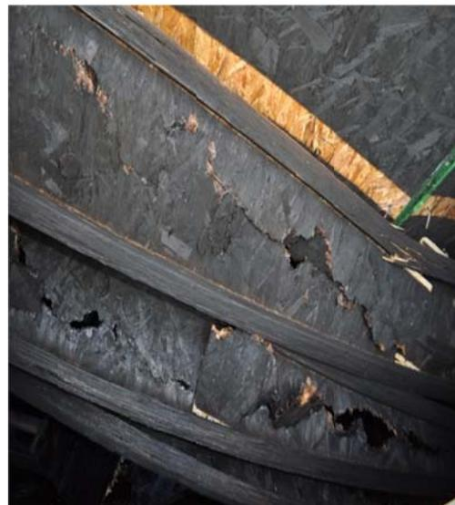
**Figure 49. Engineered I-joist Web Failure and Sheathing Separation**
