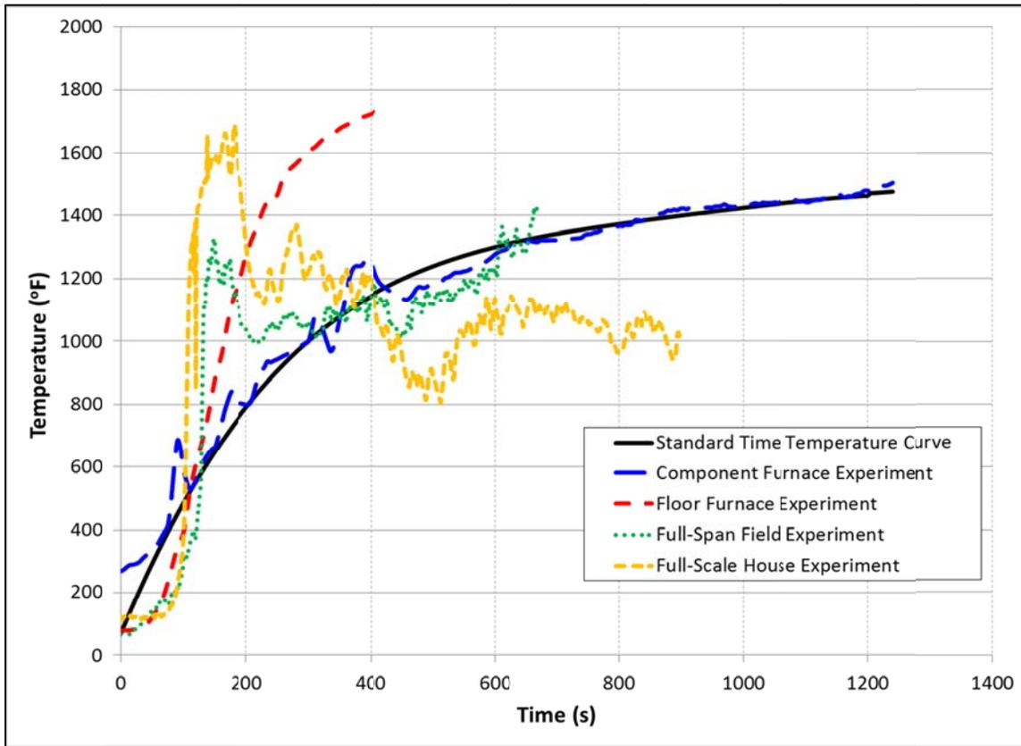
Figure 34. Comparison to the standard time temperature curve
