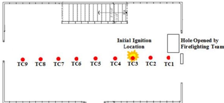
Figure 54. Experiment C Void Thermocouple and Hole Location
