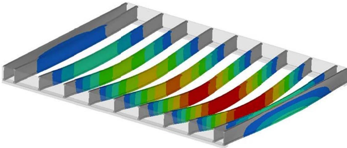
**Figure 25. Displacement contours for engineered wood I-joist supported floor assembly**
