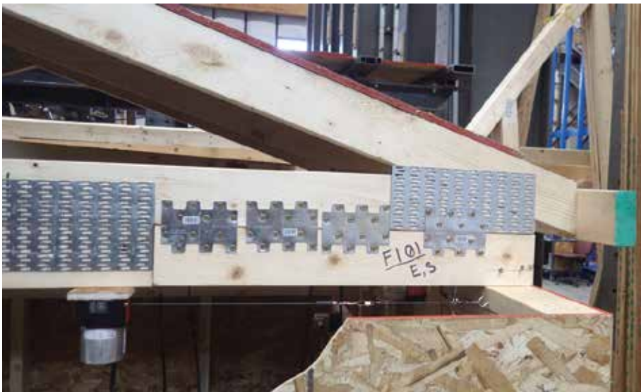
Figure 3: End view of a new SBCRI testing fixture that tests uplift and lateral loads.
