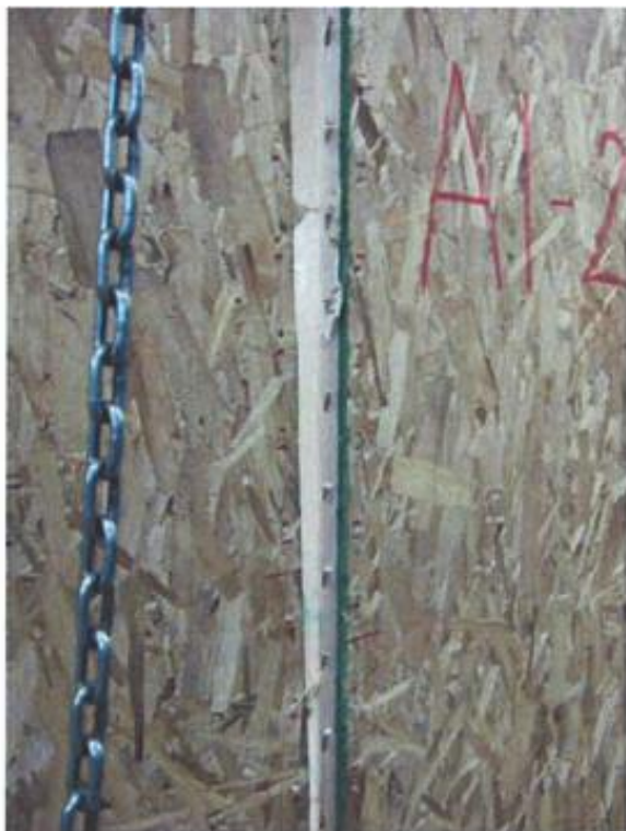
Figure 9: Typical fastener head pull-through and withdrawal for an OSB sheathed assembly
