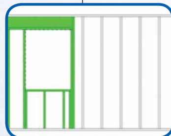
Create portal frames quickly for APA braced wall (shear panel) requirements
