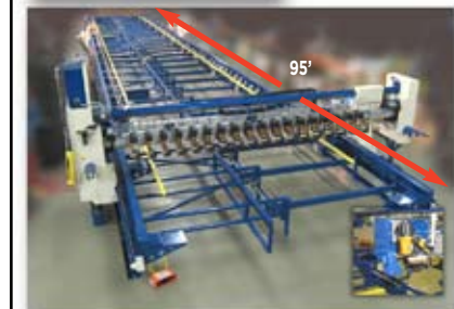
• Custom built 95 feet of expanded wall panel capability with Dual Tool Beam and Dual Top & Bottom Nailers (builds up to 76' wall)
