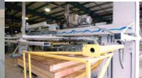
Automated Panel Stacker
