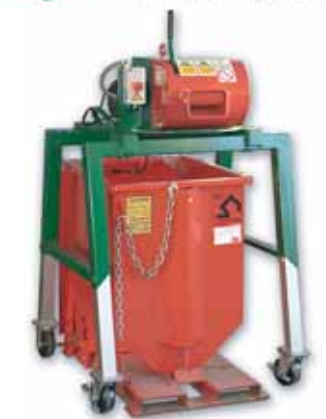
The Sweed Model 450 WM Scrap Chopper. Standard with safety infeed, "Self-Feeding" feedworks 3/4 HP drive motor. Shown with optional support stand and self-dumping hopper.
